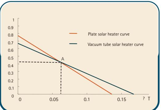
Note: The vertical coordinate stands for solar collector efficiency and the horizontal coordinate means temperature difference ratio.
